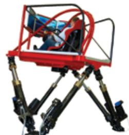
Our hexapod design enables human-in-the-loop testing and feedback of key ride and handling characteristics including ergonomic issues such as seat comfort. Recent applications include human evaluation of virtual tires and suspension designs.
