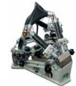
Creating and measuring forces to simulate and to test real time fatigue of the car suspensions taking into account a maximum of vehicle dynamics and creating different test loads.
