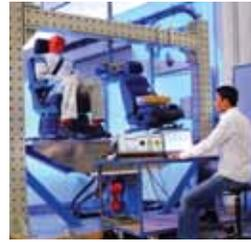
For critical analysis and test flexibility, Moog' test rigs are designed for efficient operation in a range of single- and multi-axis applications including durability, vibration, shock and performance evaluations. All units can be modified to accept a range of test specimens.
