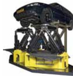
Our 6-DOF Kinematics and Compliance measurement systems have been developed in partnership with automotive manufacturers seeking highly accurate stiffness and kinematics measurements using either force or displacement control. Our revolutionary hexapod technology and electric actuation provide simpler installation, less required space and low maintenance costs. In fact, we are the only company to incorporate electric hexapod design into automotive kinematics and compliance testing.
