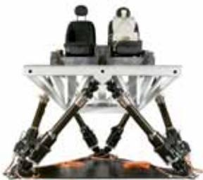
The human rated electric Simulation Table incorporates six electric actuators to deliver required 6-DOF accelerations. The hexapod design provides a minimal footprint. In addition, the test controller plays the files and provides exacting levels of control and operation to bridge the gap between digital data and human sensations.
